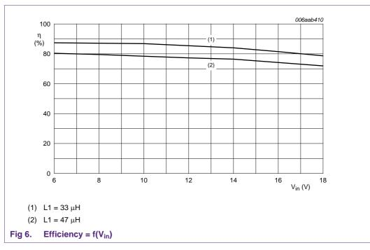
The efficiency  $P_{in}/P_{out}$  of the board as shown with L1 = 47  $\mu$ H is about 80 % for a supply voltage range from 9 V to 12 V.
